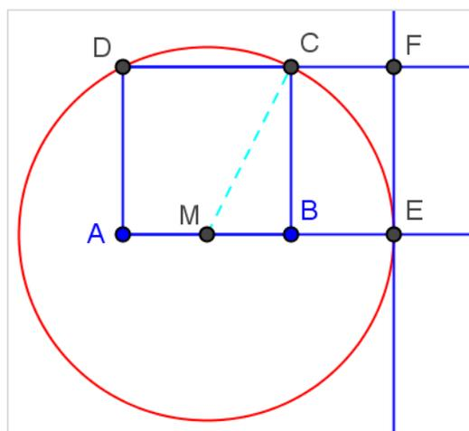
**Figure 7:** Construction of the golden rectangle using GG
